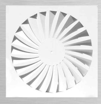
The SWF Swirl Diffuser has fixed spiral blades that create rotational as well as axial, tangential and radial air movement. This means that it produces a strong horizontal swirl, obtaining high inductivity, to allow the introduced flow to rapidly mix with the ambient air to reduce temperature and also perceived drafts or hot/cold spots.
